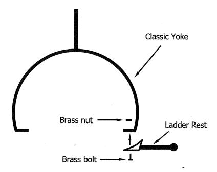
The ladder rests can be installed before the or after the Classic Yoke has been installed onto the lantern.
