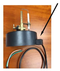
2. Install the igniter into the lantern using the 2 brass washers. Place one inside the lantern and one on the outside of the lantern. Tighten the  $90^{\circ}$  brass fitting into the bottom of the igniter. Be sure to use an approved pipe sealant. Point the valve stem to the front of the lantern.
